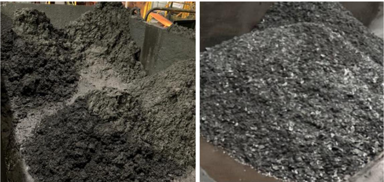
Figure 7 : Photographies de battitures
